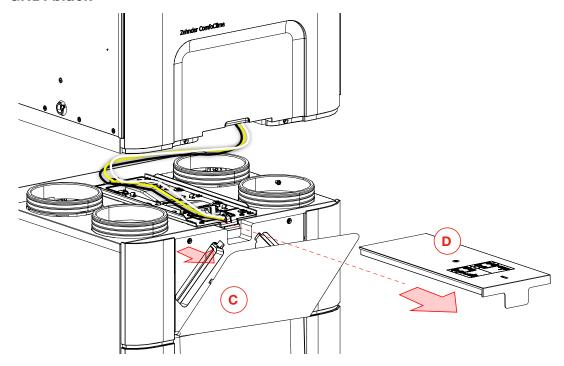
To get access to the front ComfoAir Q connector, open the black panel of the ComfoAir Q rotating it downwards and pull out the grey lid D;
